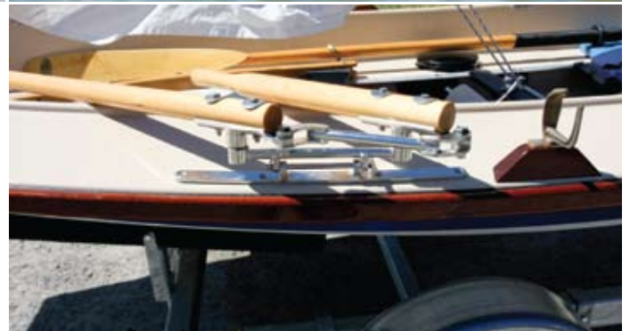
A close-up of the forward facing oar system—which allows rowers to see where they are going, instead of where they've been. It can be used on almost any kind of dinghy or rowing craft.
