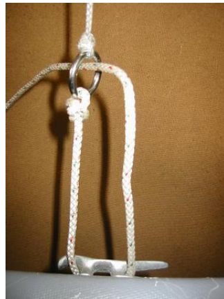
Fig. 3b: "BLOCK & TACKLE" PRINCIPLE WITH SHROUDS
